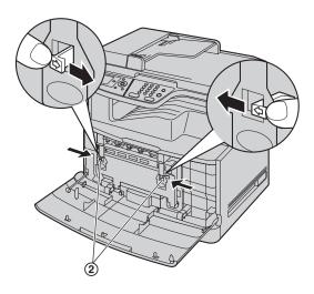
3 Lift up the levers (③) and open the drum cartridge cover (④).
